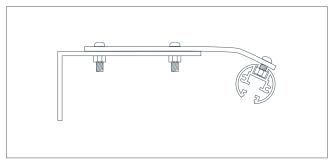
**Top brackets.** This adjustable fixing bracket is fixed to the top of the trough light and protrudes from 116mm to 204mm max.
