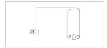
**Side brackets.** These attach to the side of the trough light and protrudes 50mm - 100mm from the wall (depending on customer specification)
